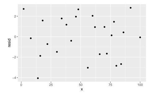
We confirm that the residuals are free from patterns. We can also plot a confidence interval of the same regression by using the geom\_smooth() layer in a ggplot:
