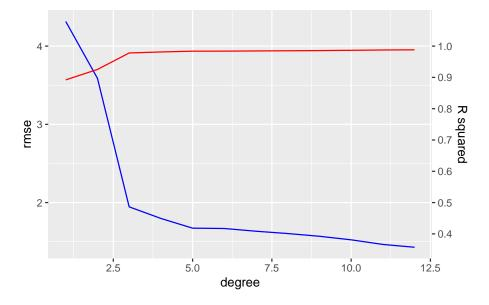
The  $R^2$  increases pretty quickly and saturates after degree 3. The RMSE decreases sharply and monothonically. It's hard to figure out the point where overfitting starts.
