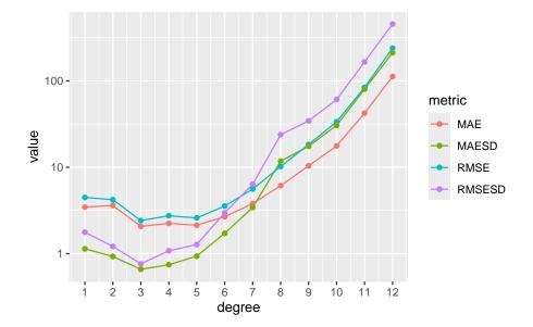
We observe that the minima of any metric happens at degree 3. This means that below that value we have underfitting, above we have overfitting (i.e. the model is loosing generality).
